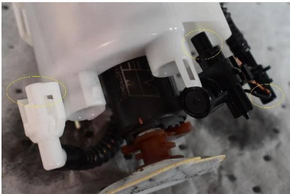
**Step 8: With the top of the housing removed from the basket, disconnect the two lines located at the bottom. There are three O-rings attached to these lines, remove them – they are no longer needed.**
