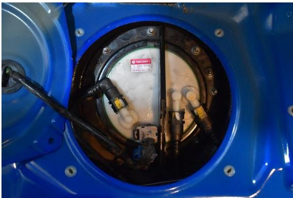
**Step 11: Install the housing back into the fuel tank. Make sure the rubber seal oriented in the right direction-it can only be installed one way. Connect the fuel lines, electrical connector and re-install the housing cover. NOTE: Improper instillation of the rubber seal, green spacer or metal bracket can cause improper seal and fuel smell in the cabin.**
