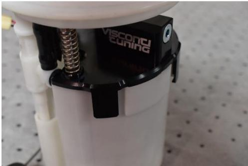
**Step 10: Insert the Visconti housing into the basket. Insure the four clips of the new Visconti housing snap into the basket. Plug in the two electrical connectors.**
