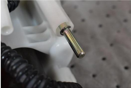
**Step 9: Remove the one c-clip located on one of the spring posts. (Fig. 5) Despite its appearance, the c-clip does have wings and will fly across your garage if not carefully removed. Set the c-clip aside for later use and separate the top and center portion of the housing. The center portion of the housing which holds your old fuel pump will not be used for later installation. Keep the top portion of the housing with springs for re-installation. (Fig. 6)**
