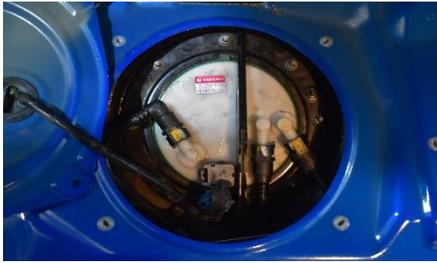
**Step 5: Remove the three fuel lines, electrical plug and eight 8mm nuts. (Fig. 2)**
